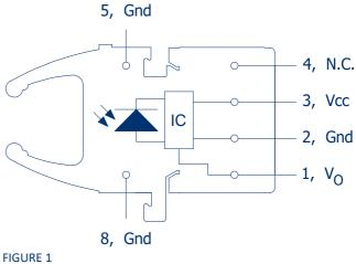
Receiver pin-out, top view
