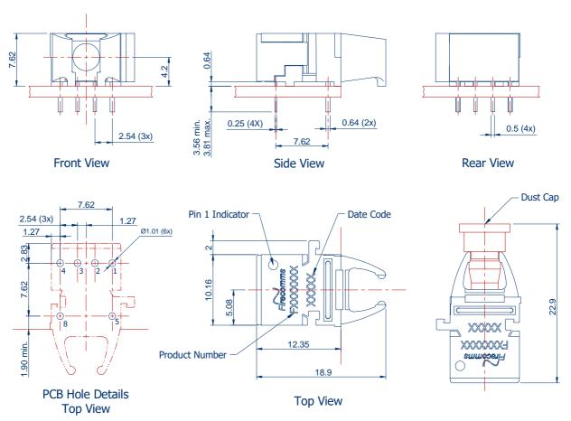
FIGURE 5 Mechanical dimensions of the horizontal receivers and PCB footprint, which is a top view General dimensional tolerance is  $\pm\,0.2$  mm
