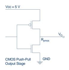
FIGURE 4 Receiver CMOS Push-Pull output stage.
