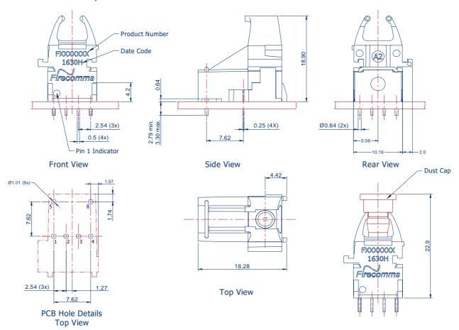
FIGURE 7 Mechanical dimensions of the vertical receivers and PCB footprint, which is a top view General dimensional tolerance is  $\pm\,0.2$  mm
